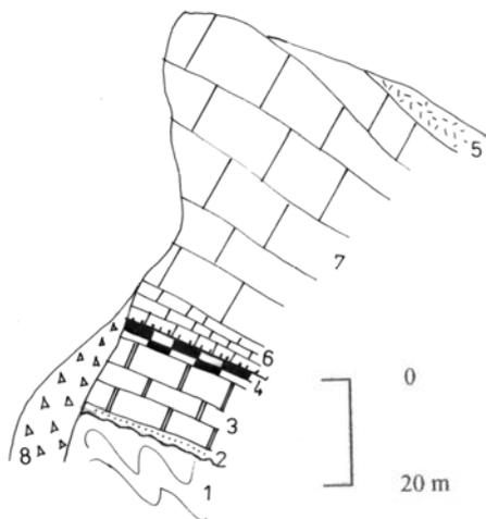
**Fig. 1.** Geological sketch of the carbonate Triassic rocks from the Piatra Șoimului klippe (under the “tourists’ balcony”, NW slope). Bucovinian Nappe: 1-crystalline basement; 2-sandstones, Seisian; 3-dolomites, Lower Anisian; 4-jaspers, Callovian-Oxfordian; 5-wildflysh, Hauterivian-Albian. Transylvanian Nappes: 6-bedded limestones, Pelsonian-Illyrian; 7-massive limestones, Ladinian - Norian; 8-limestone rubble.
