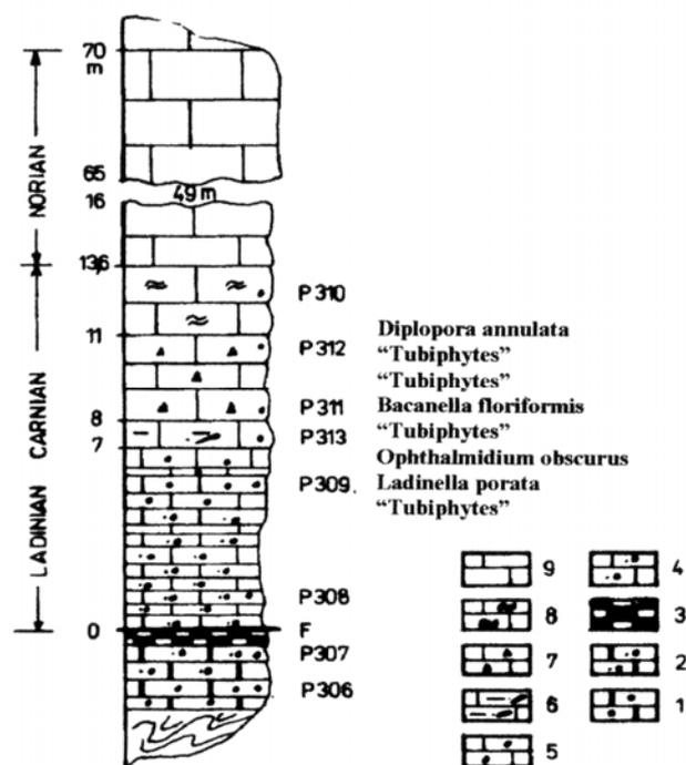
**Fig. 4.** Succession of the Triassic carbonate deposits from the Piatra Șoimului klippe (SE slope, behind the Rarău chalet) Bucovinian Nappe: 1-dolosparites, 2- dolomicrosparites, Lower Anisian; 3-jaspers, Callovian-Oxfordian. Transylvanian Nappes: 4-microsparites; 5-algal biosparites; 6-pelmicrites; 7-calcareous breccia; 8-stromatolitic limestones; 9-massive limestones; 4-9 Ladinian-Norian.
